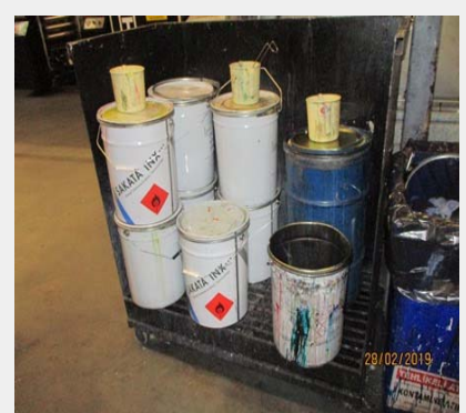
Secondary containment under chemicals
